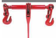
**RATCHET BINDER** - A mechanical lever device designed to tighten chain for securing a load. Due to having a gear, pawl, handle, and end fittings that screw in or out, it does not store as much energy in the handle as a lever binder does.
