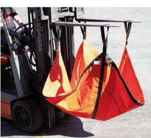
VARNING: Do not stand on, under or near a load with the sling under tension. All personnel should be alert to dangers of falling and/or uncontrolled loads, sling tension and the potential for snagging.
