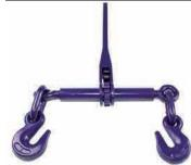
**RATCHET BINDER -** A mechanical lever device designed to tighten chain for securing a load. Due to having a gear, pawl, handle, and end fittings that screw in or out, it does not store as much energy in the handle as a lever binder does.
