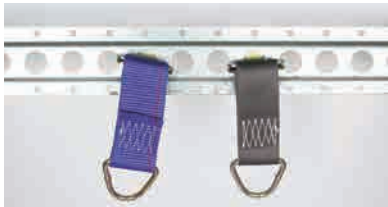
DW206 SERIES F, FIT 1" HOLE F-TRACK Length: 6" WLL: 500 LBS (227 KGS) ASSEMBLY B/S: 1,500 LBS (681 KGS)
