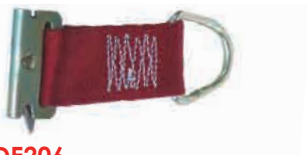
DE206 SERIES E/A, FIT E/A TRACK Length: 6" WLL: 1,500 LBS (681 KGS) ASSEMBLY B/S: 4,500 LBS (2,045 KGS)
