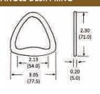
Breaking Strength: 11,000 lbs (5,000 kgs) Working Load Limit: 3,666 lbs (1,666 kgs) Weight: 0.26 lbs
