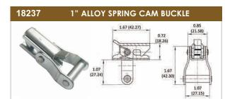
Breaking Strength: 1,500 lbs (620 kgs) Working Load Limit: 500 lbs (227 kgs) Weight: 0.15 lbs
