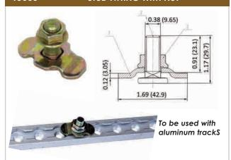
0° Vertical Breaking Strength: 5,000 lbs (2,272 kgs) Working Load Limit: 1,666 lbs (757 kgs) Weight: 0.10 lbs
