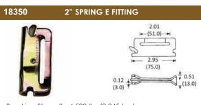
Breaking Strength: 4,500 lbs (2,045 kgs) Working Load Limit: 1,500 lbs (681 kgs) Weight: 0.19 lbs
