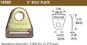
Breaking Strength: 5,000 lbs (2,270 kgs) Working Load Limit: 1,666 lbs (757 kgs)
