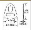
Breaking Strength: 15,000 lbs (6,800 kgs) Working Load Limit: 5,000 lbs (2,272 kgs) Weight: 0.28 lbs
